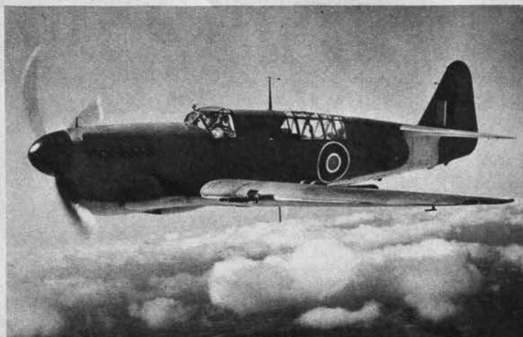
FIREFLY Long range, heavy armament mark Firefly. Low wing, built-in greenhouse, triangular tail distinguish it from inline Judy. Tailplane is set well forward.
